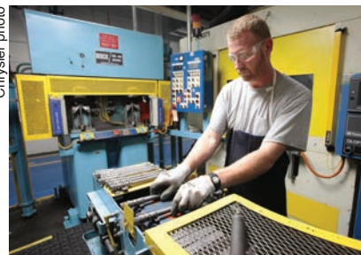
An employee at Chrysler Group's Kokomo Transmission Plant loads a transmission shaft into a polisher. The Indiana plant has been producing transmissions since 1956.
