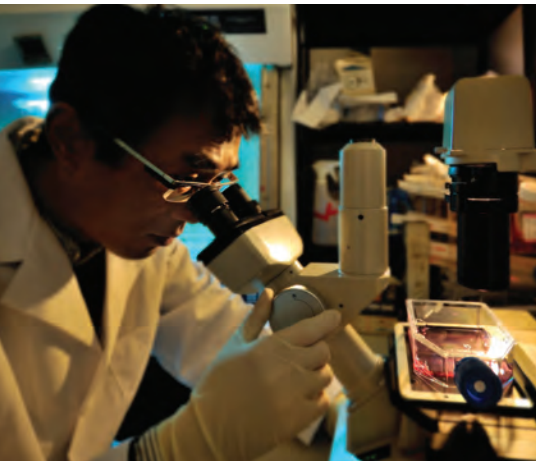
Research scientist Bin Xing uses a Nikon inverted microscope to examine brain cells in culture.
