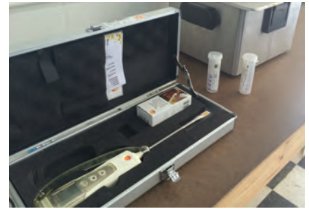
At FreshFry's manufacturing space, located in Uproar Labs, a pilot-scale fryer is in action. An oil quality tester nearby is optimizing the product performance of FreshFry's pods.
