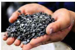
Plastic bumper covers are shredded, then processed into plastic pellets and sold to make other automotive plastic parts.
