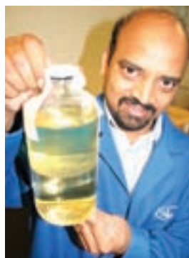
Dr. Vidya Dharmagadda, who heads the Kentucky Department of Agriculture's motor fuel and pesticide testing laboratory, shows a fuel sample that is fuel on top and water on the bottom.
