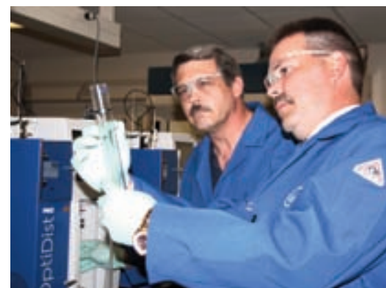
Commissioner Farmer, right, and Tom Bloemer, manager of the Weights and Measures Inspection Branch, examine the recovery column of a gasoline and diesel distillation testing instrument at the new motor fuel testing laboratory in Frankfort.
