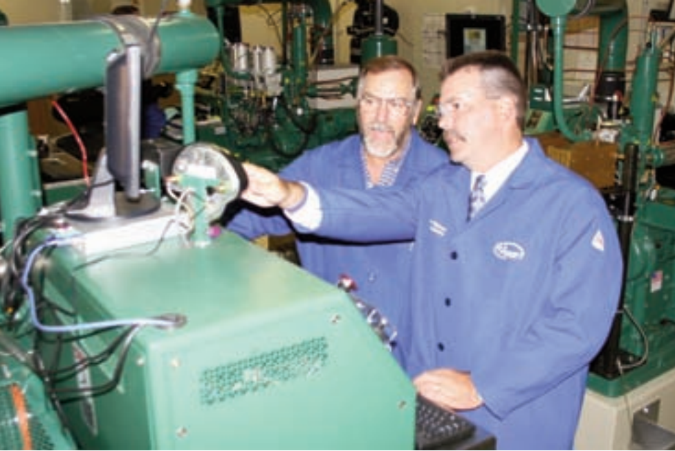
Commissioner Farmer, right, and Bill Day, an employee in the motor fuel lab, observe a special four-cylinder engine that enables technicians to measure octane in motor fuel.
