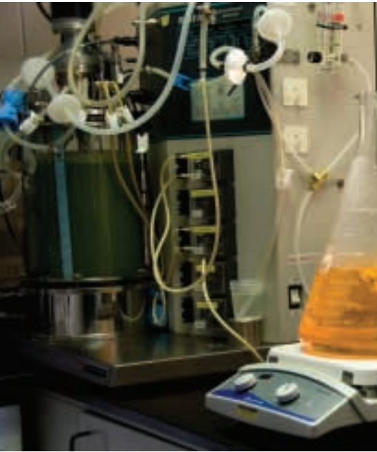
An example of an Alltech Algae research fermentor in the pilot plant used for the development of new processes.
