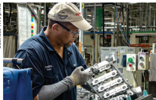
Henry "Sonny" Smith, a Toyota West Virginia team member for 17 years, inspects the cam housing on a four-cylinder engine.
