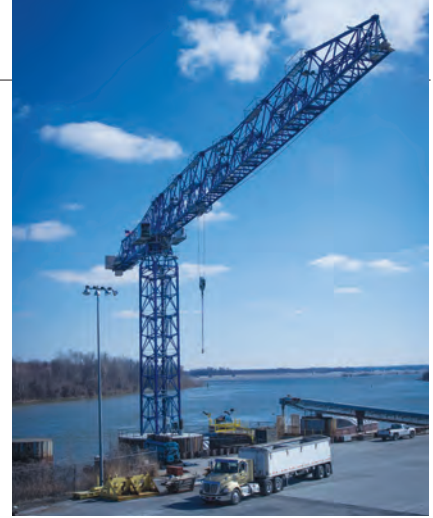
High capacity tower cranes such as this Linden Comansa 30LC1450 recently erected in Paducah, Kentucky are helping busy ports like the Paducah/McCracken County Riverport Authority deal with today's vessel traffic and be ready for tomorrow. The crane's addition furthered the Riverport capabilities in international shipping and receiving and was cited in its application for Foreign Trade Zone designation.
