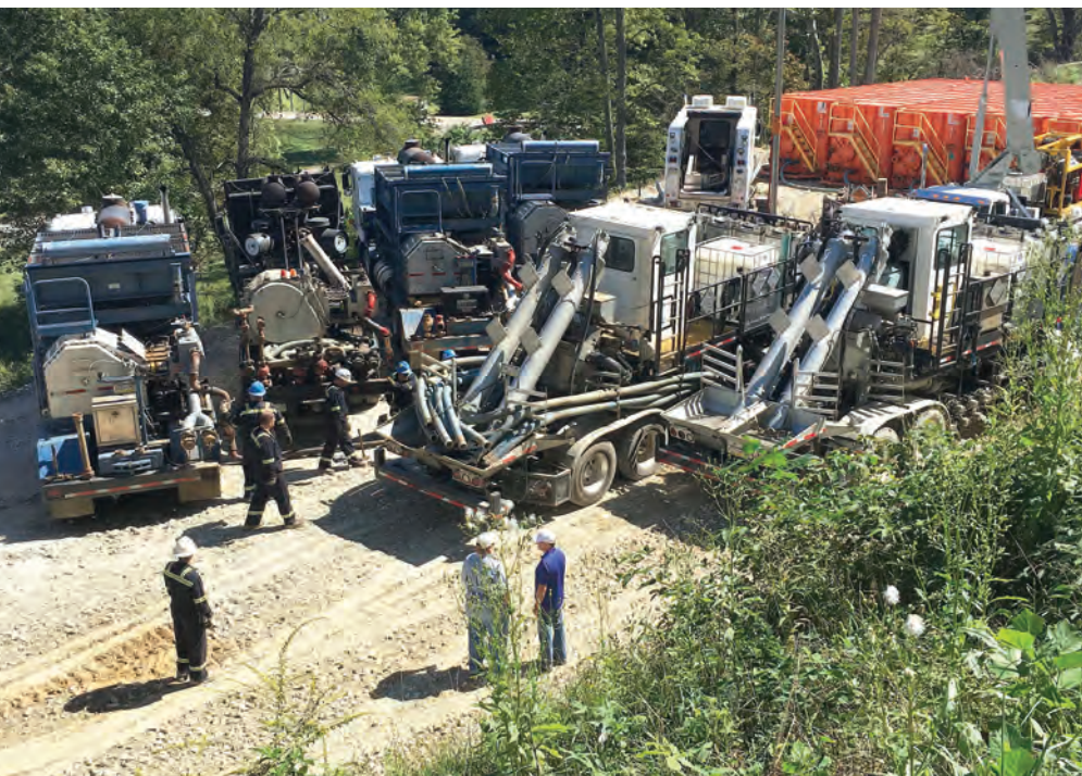
Well operators position pump trucks around the well bore prior to “fracking” the BlackRidge 3Ds #1-HOR well in Lawrence County. The red storage tanks hold the water used in hydraulic fracturing process.
