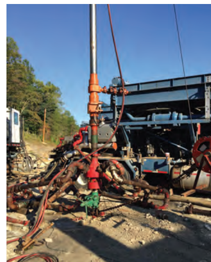
Wellhead equipment is used to connect the pump trucks and sand blending equipment to a well during a hydraulic fracturing well stimulation.
