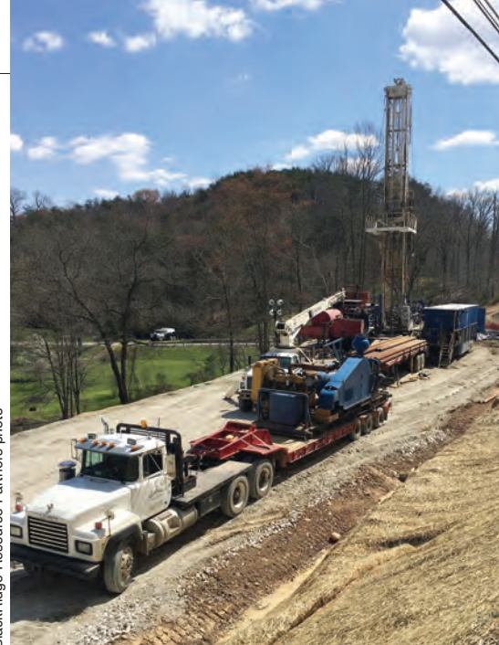
Workers from BlackRidge Resource Partners rig up a drill on the #1-HOR well located in Lawrence County
