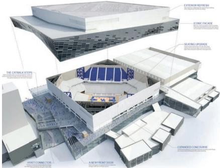
A three-dimensional infographic depicts the planned interior and exterior details of Rupp Arena. Construction began in 2018 on a new 100,000-s.f. Lexington Convention Center and is expected to be complete in 2022.
