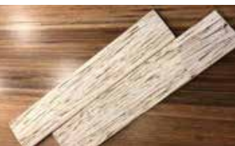
Fibonacci's patented HempWood, made from hemp fiber and soy-based adhesives, can be used in a wide variety of products.
